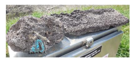
Leachate scale samples prior to installing the FlowMark submersible system in manhole number 11. The 8" gravity main collection pipe would scale completely closed in two months requiring frequent hydro-blasting and acid cleaning.
