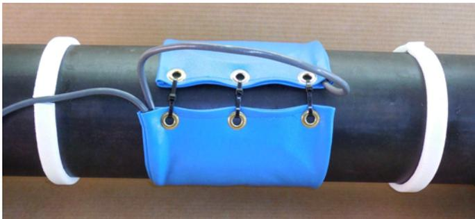
Install treatment pads opposing each other using 6 cable ties provided. Mark the pipe and install weather stripping.
